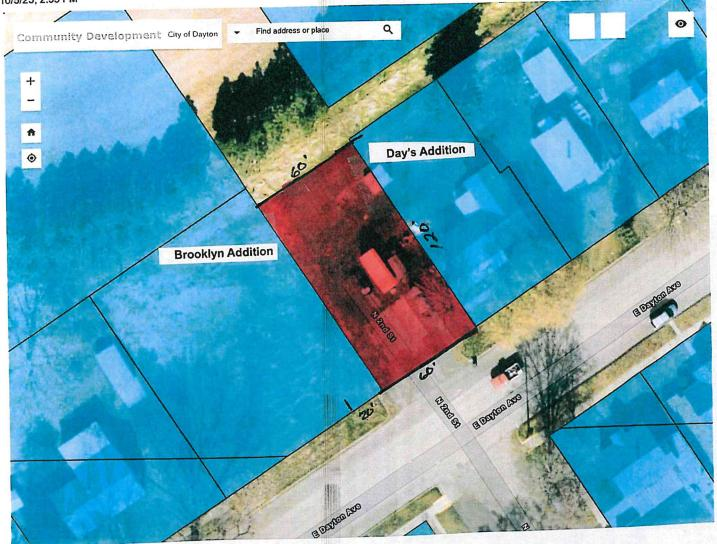
VACATING CITY RIGHT-OF-WAY LOCATED IN DAY'S ADDITION OF DAYTON, NAMELY, ALL THAT PORTION OF THE (60FTX120FT) RIGHT-OF-WAY DISCRIBED AS FOLLOWS, BEING A PORTION OF THE NORTH 2<sup>nd</sup> STREET RIGHT-OF-WAY NORTH OF EAST DAYTON AVENUE LYING WEST OF BLOCK 68 OF DAY'S ADDITION TO DAYTON AND EAST OF BLOCK 60 OF BROOKLYN'S ADDITION TO DAYTON. CONTAINING 7200 SQ. FT. MORE OR LESS.
