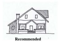
Dormer scale is subordinate to main roof mass, side extension is a continuation of roof slope.
