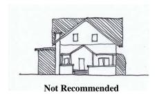
Dormers are oversized and not scaled subordinate to the primary roof mass, side extensions have different roof slopes from the main roof.
